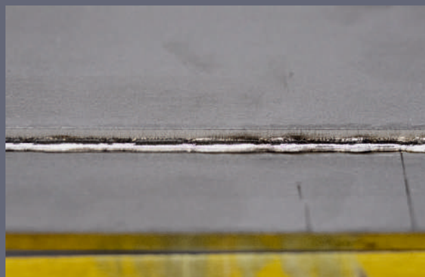
WELDING OF STEEL WITHOUT FILLER METAL
